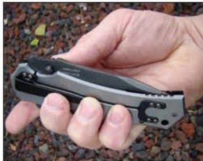
Thumb opening of the M1 requires gripping the handle with the fingertips on the dip. Gripping too tightly on the lock bar can apply pressure to the detent and bind the blade.
