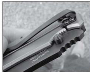
This close-up shows how the overtravel tab of the dip acts as a stop for the frame lock.
